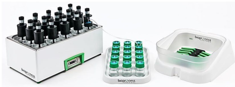
Figure 1. Photo of AMPTS (II) apparatus.
